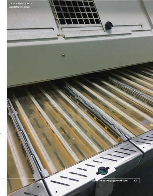
Remember, only IR dryers can be used for this type of control as we need a quick response in changing power based on the temperature sensor reading. The target is to maintain a constant board temperature. That temperature should be high enough to allow a quick evaporation of the water from the ink but it needs to be low enough to avoid evaporation of water from the substrate.
