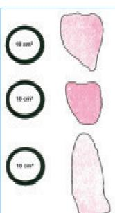
blot. Dividing the volume of ink applied by the area measured for the blot gives an indication of the ink film thickness available on the surface of the roll. It is claimed that this system is inaccurate because of the human effect on the amount of ink applied, the doctoring of the ink and the measuring of the blotted area.
