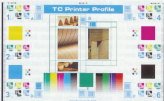
Figure 2: Five colour test forme. Only barcodes in cyan are used.
