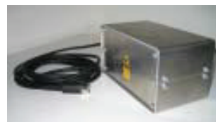
Figure 6: The device used for measuring the surface profile as shown in figure 2, 3 and 4 was developed, designed and built (including software) by Technology Coaching BVBA. Measuring resolution < 4 µm.
