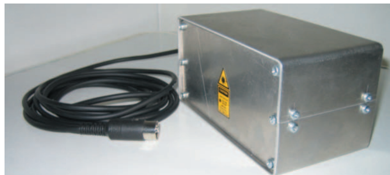
Figure 6: The device used for measuring the surface profile as shown in figure 2, 3 and 4 was developed, designed and built (including software) by Technology Coaching BVBA. Measuring resolution <4 µm
